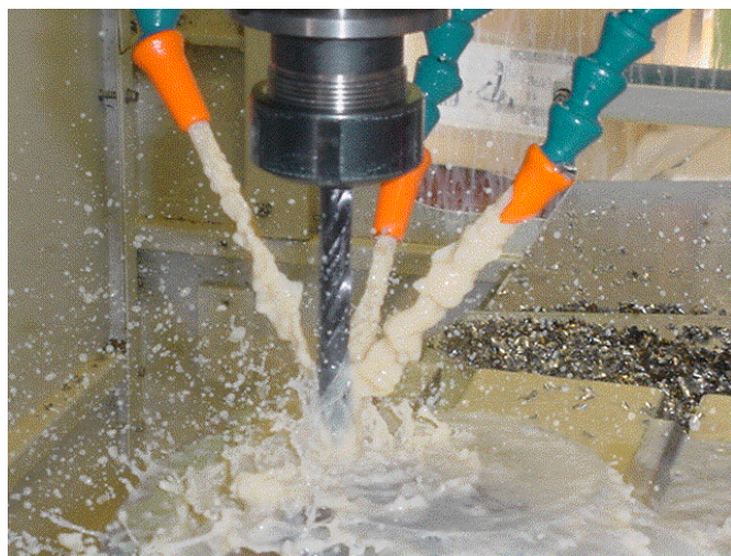
Figure 5. Application of the cutting fluid by flooding over the tool-workpiece.
