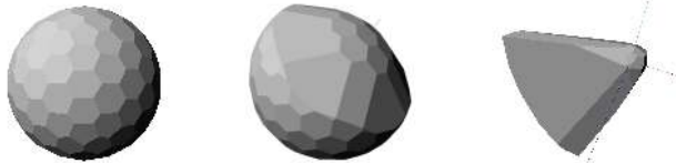
Figure 3. Discrete Wulff shapes, from left to right: isotropic, preferring one main direction, more complex shape that penalizes a segment of normals much more strongly than the rest.
