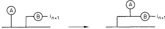
Fig. 27. The last operation in which i_{n+1} participates must be of this form
