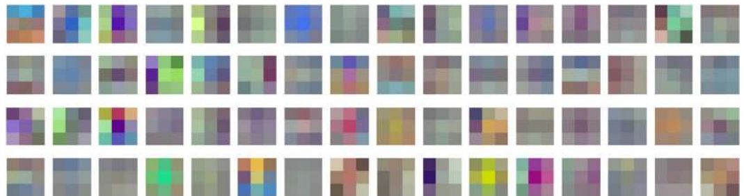
Figure 3. The visualization of 64 filters of the first convolution layer in the VGG-16 model. Filters with 3 \times 3 \times 3 dimensions are projected into pixel space for the visualization.
