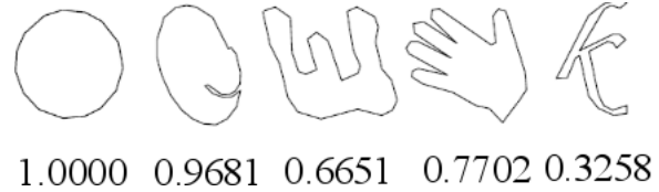
Fig. 5. Graphical representation of convexity (Zunic and Rosin, 2002).
