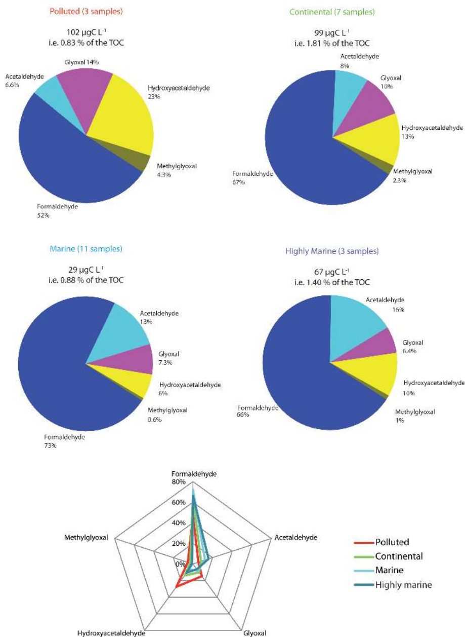
Fig. 7. Distribution of carbonyls (formaldehyde, acetaldehyde, glyoxal, methylglyoxal, hydroxyacetaldehyde) as a function of air mass categories (percentages are calculated using concentration in \mu\text{M} ). On the left-hand side, the sum of the concentrations of these compounds in \mu\text{gC L}^{-1} is indicated as well as the percentage obtained by comparison with the TOC. The radar chart shows the relative contribution of each compound as a function of the air mass category.
