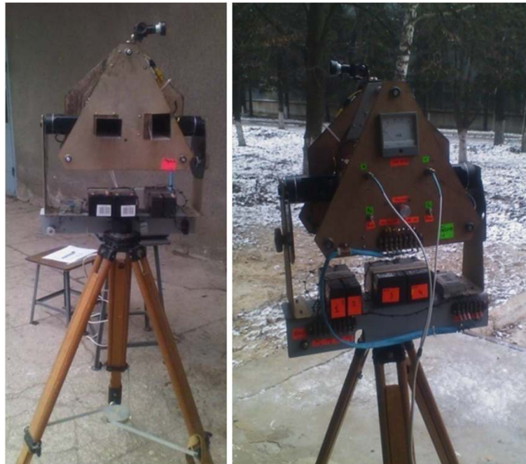
Figure 2 Ground surveillance radar system used for experimental data collection. Wavelength—8.8 mm, emitted radar power—15 mW; receiving/transmitting antenna beam width in both E and H planes—60°; level of side lobes in horn antenna pattern—24 dB; cross-polarization level \leq -30 dB; receiver noise figure—20.2 dB; two-channel 16 bit ADC; and sampling rate in digital records—8 KHz.
