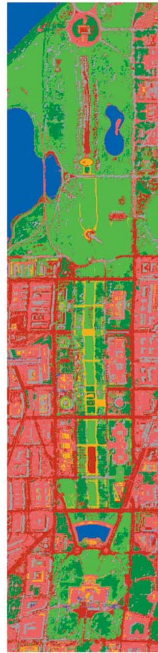
Fig. 13. Washington, DC data. A classification map for obtained by applying a neural network classifier on an extended morphological profile with two PCs, four openings, four closings, and nonparametric weighted feature extraction. The neural network classifier was applied to 14 NWFE features. The overall accuracy of the test data was 98.5% in this case.
