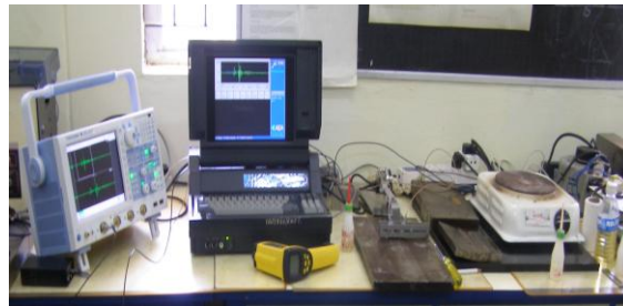
Figure 1 . TOFD Experimental Set Up.
