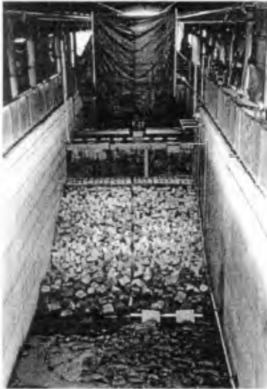
Figure 3. Front View of Model Breakwater With Vertical Wall in the GWK
