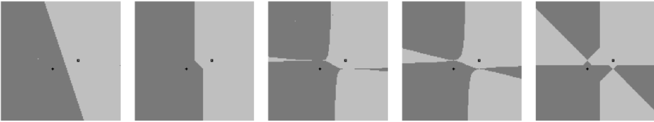
Fig. 1. The Voronoi diagram for two points using, from left to right, p -distances with p = 2 (Euclidean distance), p = 1 (Manhattan distance, which is still metric), the nonmetric distances arising from p = .5 , p = .2 , and the min (1-median) distance. The p -distance between two points (x_1, y_1) and (x_2, y_2) is: (|x_1 - x_2|^p + |y_1 - y_2|^p)^{1/p} ; the min distance is \min(|x_1 - x_2|, |y_1 - y_2|) . Min distance in 2D is illustrative of the behavior of the other median distances in higher dimensions. The region of the plane closer to one point is shown in dark gray, and closer to the other in light gray. Note that only the first is invariant to our choice of axis direction.
