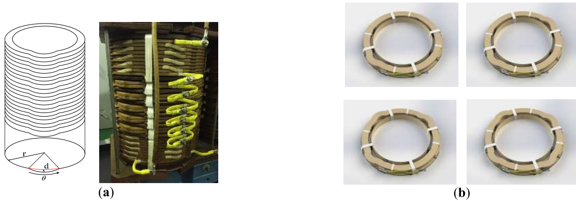
FIGURE 1. Diagrammatic sketch of winding RD fault: (a) diagram and image of RD; (b) 3D visualization of winding RD with faults manufactured at different directions.
