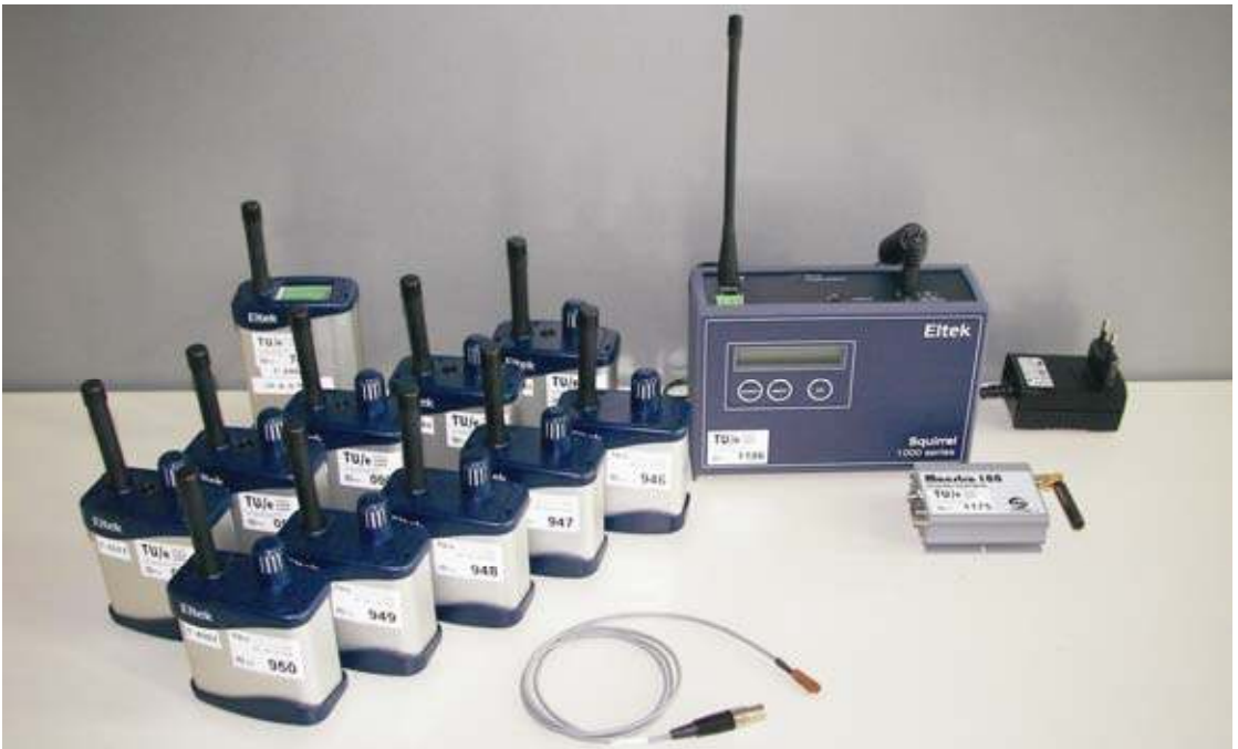
Figure 2.3: Permanent measurement equipment: Eltek datalogger, 10 Eltek T and RH transmitters, 1 Eltek mV transmitter, 1 Maestro GSM modem and a surface temperature sensor (to connect to a transmitter).
