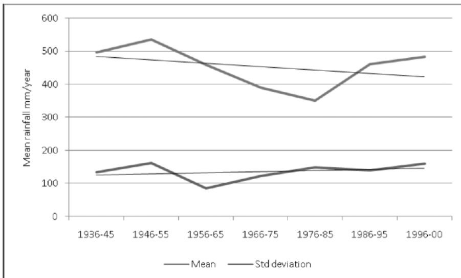
Figure 5.7—Decadal mean and variability of annual rainfall, Madoua station (Sahel zone, Tahoua region), Niger
