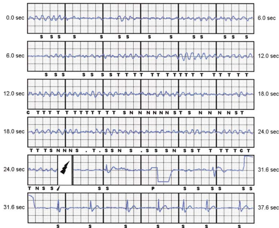
Figure 4 Subcutaneous implantable cardioverter–defibrillator electrogram of ventricular fibrillation from patient 10. Ventricular fibrillation (VF) onset occurred 2 s prior to this recording. Charging begins 14 s after VF onset. Subsequent inaccurate classification begins to occur 2 s later, partly due to fine noise not apparent on visual inspection. The majority of sensed events during the next 11 s are not classified as tachycardia, further delaying therapy until 26.8 s after VF onset (shock indicated with lightning symbol). C indicates onset of charging when first seen and commitment to shock delivery when seen a second time. N indicates sensing of an event which is classified as noise. S indicates sensing of a ventricular event not classified as tachycardia. T indicates sensing of a ventricular event classified as tachycardia. A dot indicates sensing of an event which is unclassifiable.
