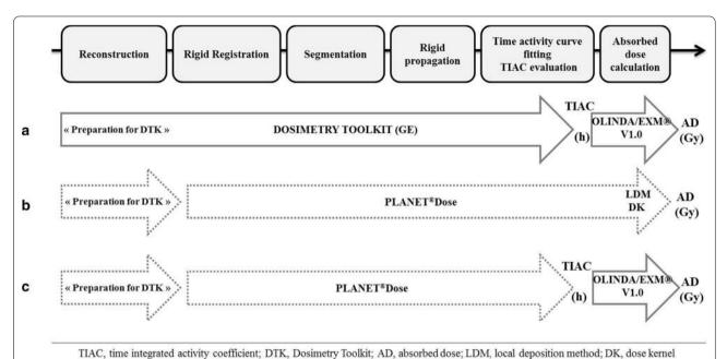
Fig. 2 Dosimetry workflow using the reference dosimetry approach Dosimetry Toolkit + OLINDA (a) and the PLANET® Dose package with the LDM and DK methods (b). The PLANET® Dose + OLINDA approach (c) was used to evaluate independently the AD calculation methods
