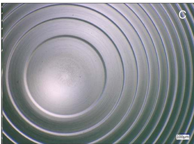
Figure A. Microscopy pictures of the intraocular lens (IOL) surface: (A) extended depth of focus IOL; (B) trifocal IOL; and (C) bifocal IOL.
