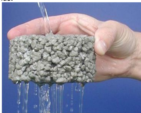
Figure 1. Sample of permeable concrete (1)
