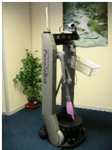
Fig. 1: The PeopleBot™ robot fitted with arm and hand. This robot was used in the children's study.
