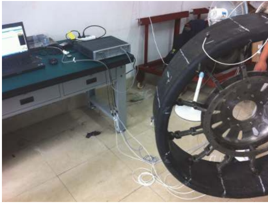
Fig. 7. Vibration modal test
