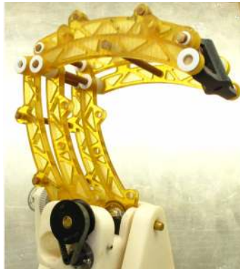
Fig. 7 Photograph of the remote center of motion (RCM) linkage portion of the DBS insertion mechanism that couple to the above-mentioned translational motion base.
