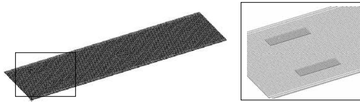
Fig. 4. Finite element model of an actively controlled cantilever plate.
