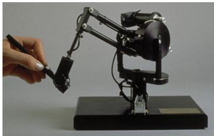
Figure 3. PHANToM TM haptic interface (Image courtesy of SensAble Technologies, Inc.)
