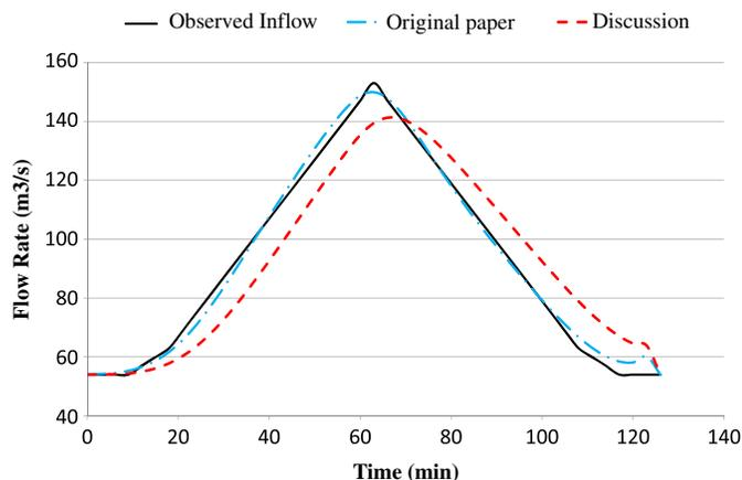
**Fig. 1.** Comparison of routed upstream hydrographs of the original paper and the discussion for triangular flood data.
