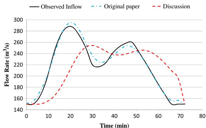
**Fig. 2.** Comparison of routed upstream hydrographs of the original paper and the discussion for double-peak flood data.
