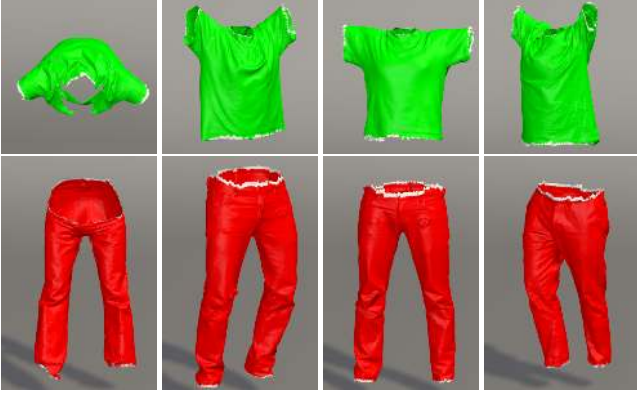
Fig. 7. Segmentation results: rows of scan geometry segmentations, shirt (top row), pants (bottom row). After solving the discrete MRF on the body topology we propagate the obtained labels back to the scan. This results in segmented scans \mathcal{S}_k . Boundaries (shown in white) can be easily identified and are propagated to the scans. Such labels provide important information for the multi-cloth alignment step. They allow ClothCap to estimate consistent geometry with smooth boundaries.
