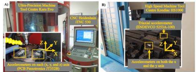
Fig 6. Detail of the micromachining center and devices.
