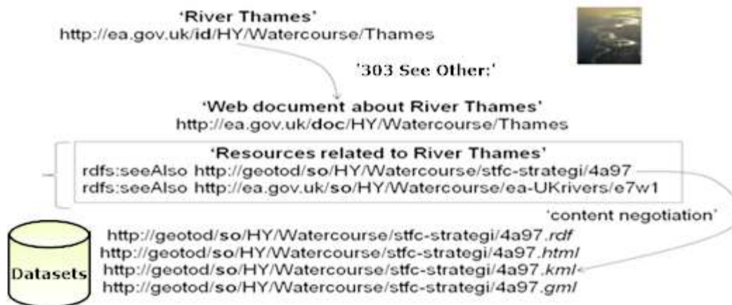
Figure 8: Use of HTTP URIs and RDF vocabulary to identify, expose and link related Web-based resources.
