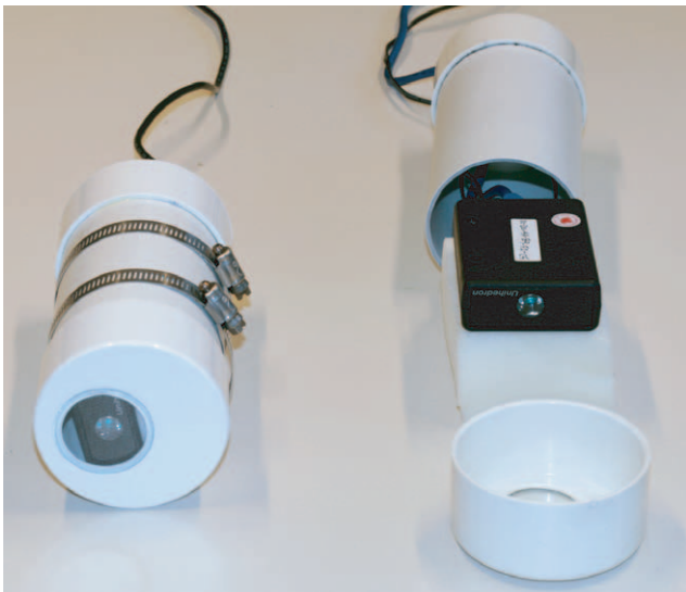
Figure 2. Photograph showing the Sky Quality Meter installed in its protective housing (SQM-LU left), along with an expanded view (SQM-LE right). The housing at left is shown with the two included hose clamps that allow easy attachment to a stake or pole. The USB version (left) requires only one cable, but at the cost of shorter cable runs and the internal heating provided by the Ethernet version (right).
