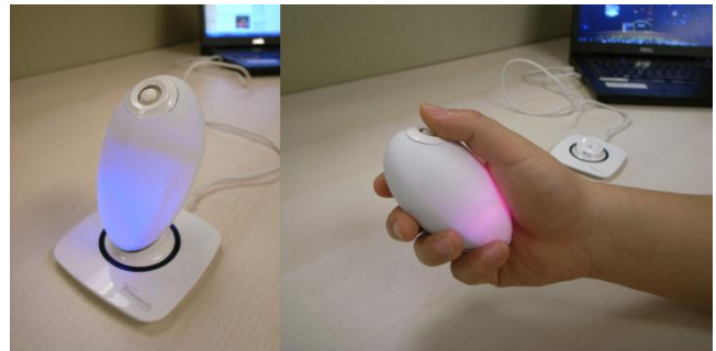
Figure 1: The core of cloud mouse is inertial sensor and haptic sensor. While pointing, users can squeeze cloud mouse to hold virtual object in display.
