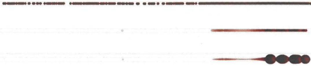
Fig. 2. Step-by-step construction of a single CloudLine. ( top ) A sequence of event data on a linear timeline, where each event is represented by a circle. It is practically impossible to distinguish between the high and low density areas. ( middle ) The same sequence after mapping the importance function to opacity of each circle. Importance function is described in Section 4. The change in opacity levels shows the structure of the sequence better. However, overplotting and the fact that maximum opacity can be reached very quickly don't allow for finer details in high density areas to be shown. ( bottom ) Importance function mapped to both opacity and size of the circles. Several event episodes can be identified much more easily.
