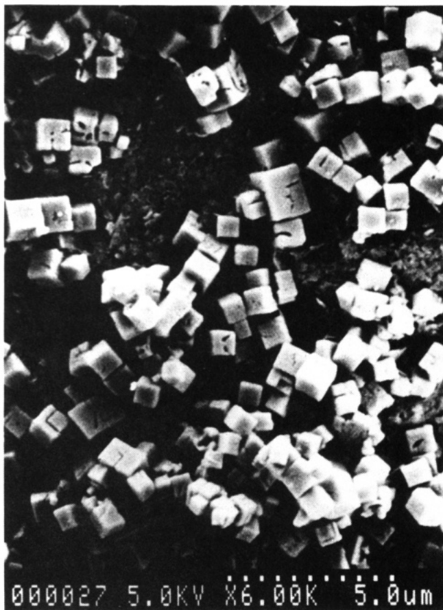
Figure 1. SEM data for as-synthesized cubic cloverite.
