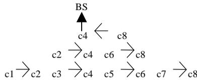
Fig.2 Data gathering in a chain-based binary scheme
