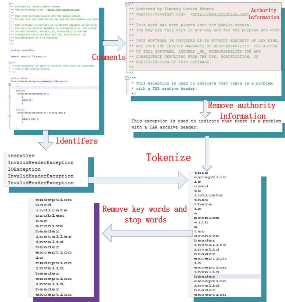
FIGURE 3: The process of preprocessing the class InvalidHeaderException.java in jEdit .
