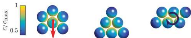
Fig. 1 Stable planar arrangements of N = 6 attracting phoretic particles. Colorbar shows the relative surface concentration. The asymmetry of the geometry sets whether the cluster translates (left) remains stationary (center) or rotates (right).
