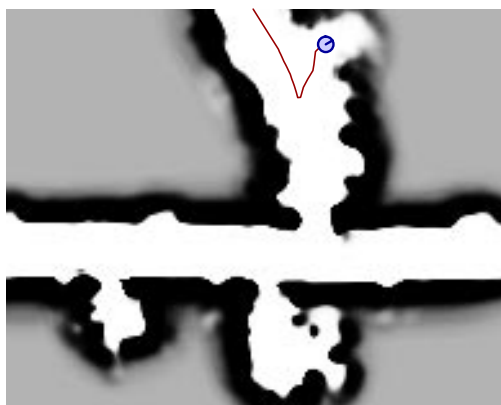
Figure 16: Failure anticipation after learning to recognize closed doors. The robot turns around much earlier.
