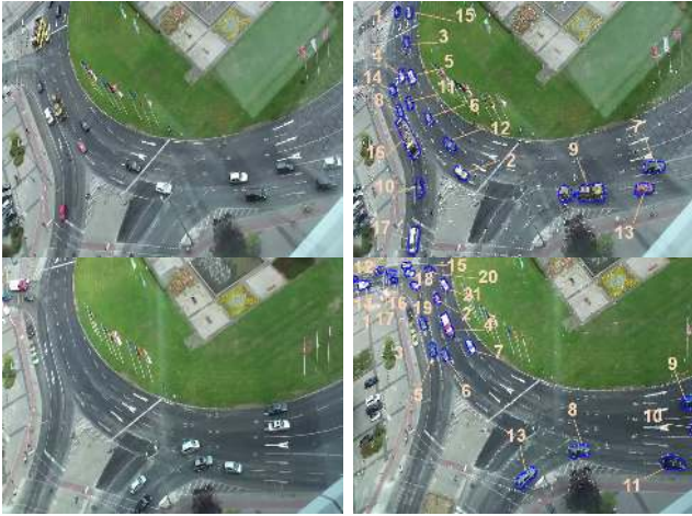
Figure 5. Top: (a) First frame and the annotated motion segmentation of the frame 153 from a static camera. Bottom: (b) First frame and the annotated motion segmentation of the frame 153 from a hand-held camera.
