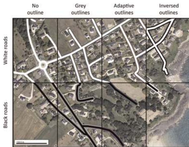
Figure 6. Adaptive colour contrasts between roads and orthoimagery
