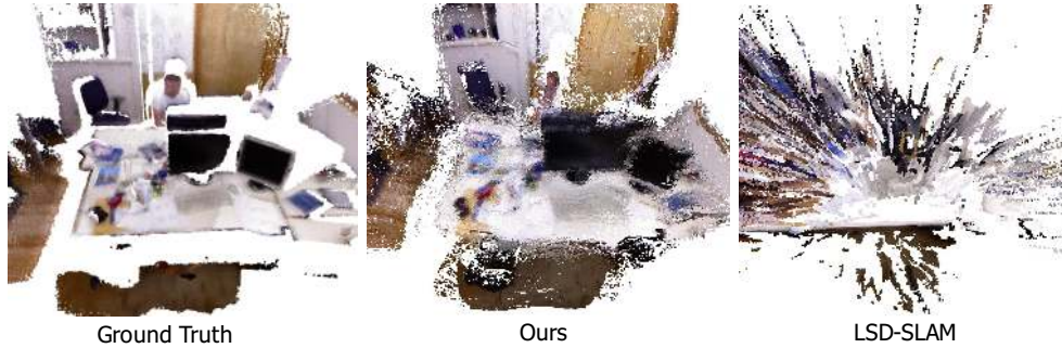
Figure 5. Comparison on a sequence that includes mostly pure rotational camera motion between the reconstruction obtained by ground truth depth (left), proposed method (middle) and LSD-SLAM [4] (right).
