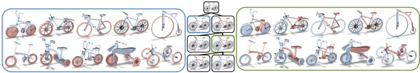
Figure 1: Structural co-hierarchical analysis of a set of velocipedes (bicycles, tricycles and four-cycles). The resulting co-hierarchy (center) is illustrated by a single sample shape from the set, where each node represents a part assembly. Two of the nodes (highlighted in blue and green) are expanded to show the insight gained by the analysis which relates parts with rather different geometries but similar functions.
