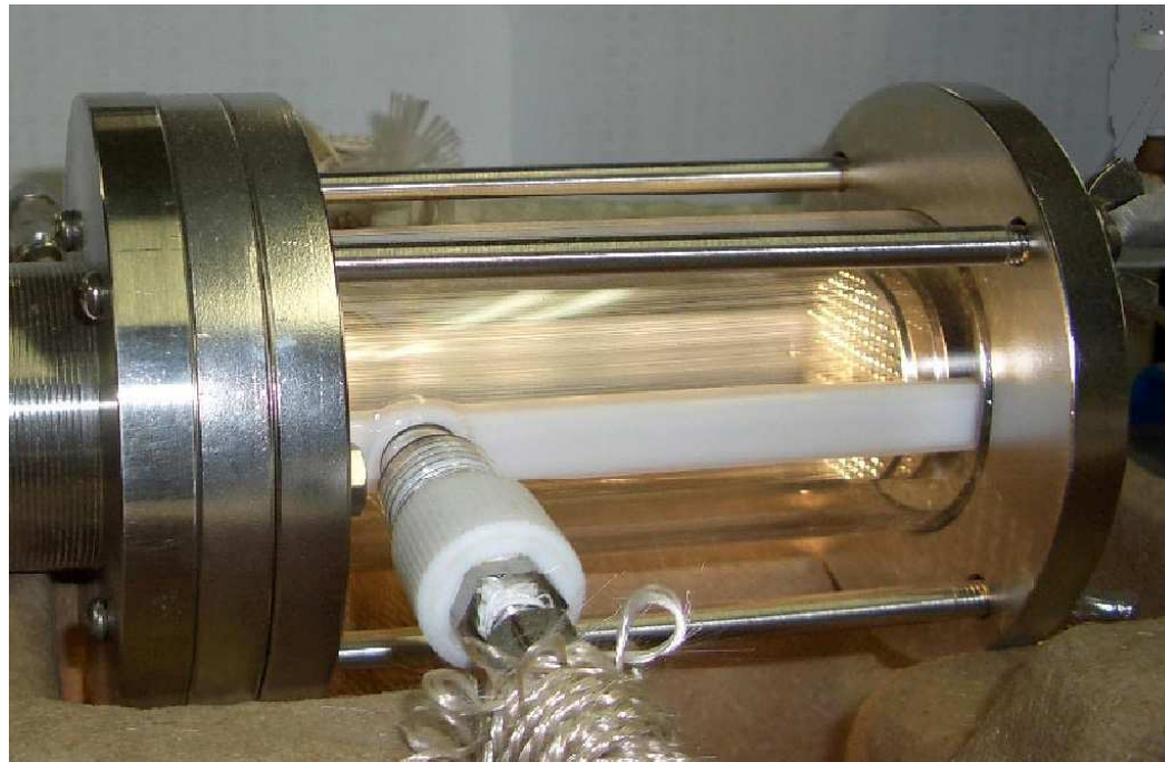
Fig1: optical-fiber reactor with light irradiation
