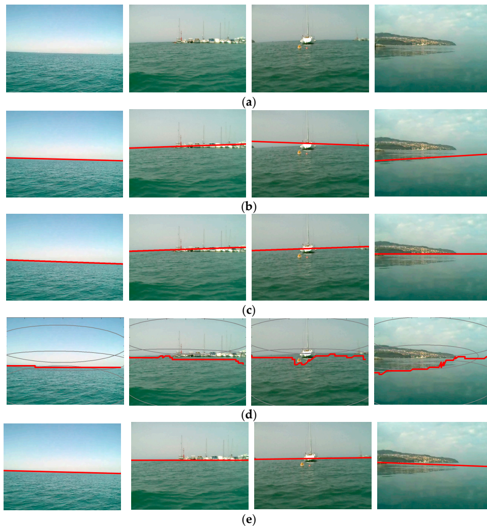
Figure 12. A comparison of various horizon line detection methods using MODD: (a) Original image; (b) Wang's algorithm; (c) MSCM-LiFe; (d) SSM; (e) CFS method.
