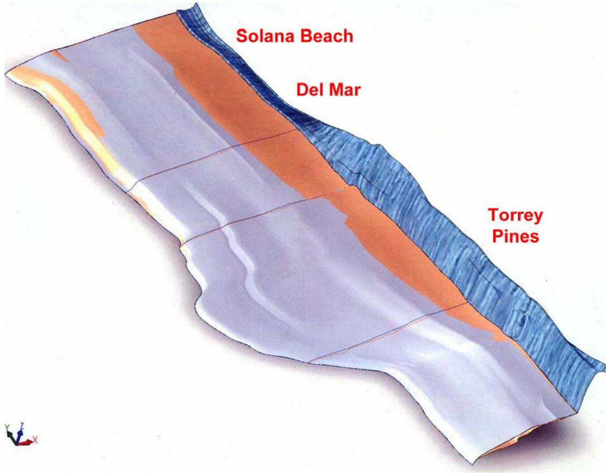
Figure 57: Three-dimensional Torrey Pines Sub-Cell forecast of sediment (gray) and bedrock (brown) surfaces from CEM simulation at time t = 56 yr forward from initial condition in Figure 56.
