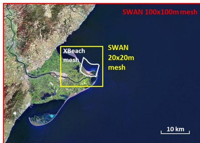
Figure 4. Location of the computational meshes used to run SWAN (red, coarse mesh; yellow, fine mesh) and XBeach (white, local mesh) models. Modified from ICGC ( http://www.icgc.cat/vissir3/ ).
