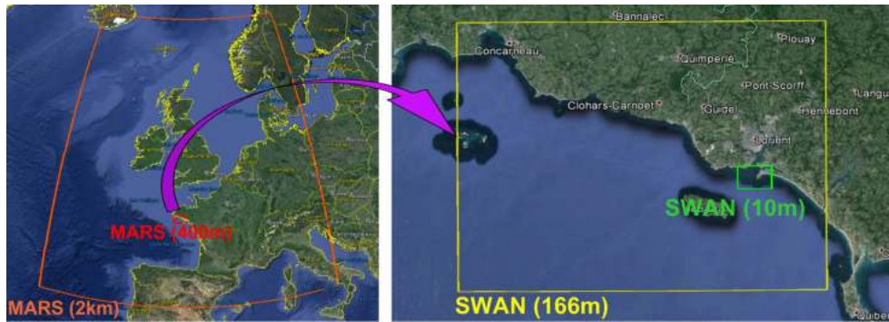
Figure 2. Location map of Gâvres, areas covered by the regional and coastal simulations (sea water level with MARS on the left, wave characteristics with SWAN on the right).
