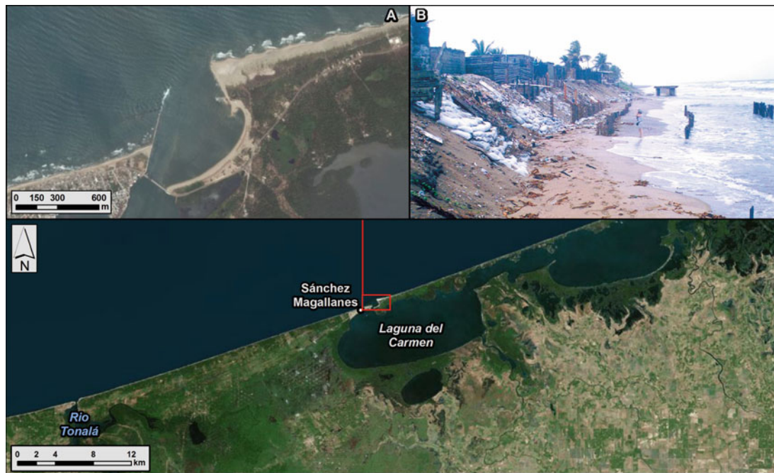
Figure 6.61. Shoreline offset at the Laguna del Carmen jetties at Sánchez Magallanes illustrating net west-directed longshore sand transport (A; Image credit: Microsoft Bing Maps Aerial). Down-drift beach erosion west of the jetties has resulted in significant property damage (B; photo from Hernández-Santana et al. 2008, used with permission).
