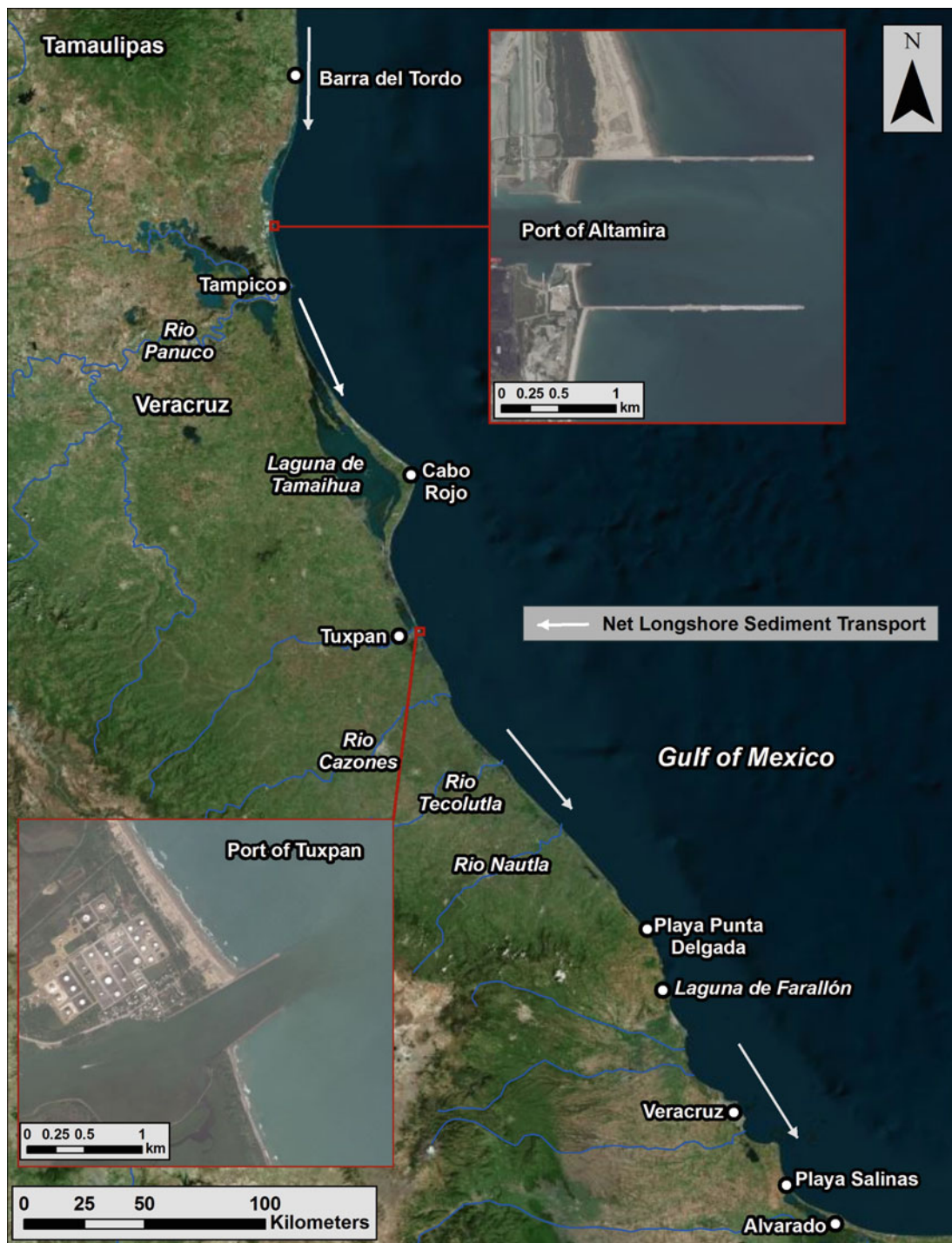
Figure 6.59. Veracruz Neritic shoreline between Barra del Tordo and Playa Salinas illustrating a net south-directed longshore transport system. White arrows show the direction of net littoral sand transport. Image credit: Microsoft Bing Maps Aerial.
