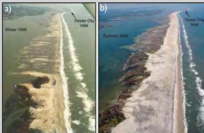
Box Figure 3.2c North oblique photographs of northern Assateague Island in 1998 after a severe winter storm. The left photo of Assateague Island barrier shows clear evidence of overwash. The right 2006 photo shows a more robust barrier that had been augmented by recent beach nourishment. The white circles in the photos specify identical locations on the barrier. The offset between Fenwick Island (north) and Assateague Island due to Ocean City inlet and jetties can be seen at the top of the photo. Photo sources: a) National Park Service, b) Jane Thomas, IAN Photo and Video Library.
