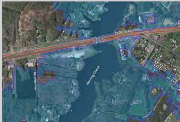
Box Figure 9.3c Sea-level rise in 2100 using present day sea-level trends coupled with a category 2 hurricane storm surge.
