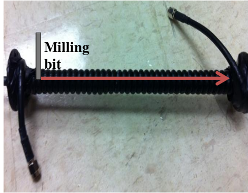
Figure 3.6. Image of a coiled coaxial cable resonator.
