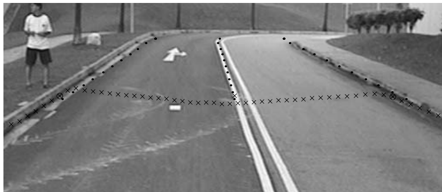
Figure 4: Road surface image and corresponding range points (crosses) recorded from a SICK TOF LADAR.
