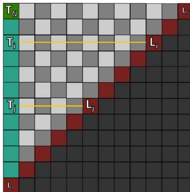
Figure 4. Two-dimensional dynamic programming matrix underlying the algorithm of the non-comparative part of COBOLD. Both axes correspond to an input sequence of length L . Each T_i = (1, i) entry in this matrix corresponds to the optimal RNA structure S_i that is co-transcriptionally formed for a sub-sequence L_i , L_i \leq L , of the original input sequence. By starting the traceback procedure at field T_i = (1, i) of this matrix, we can retrieve S_i by subsequently following the structural information stored in each subsequent node, which also points to the following one in the path. At the end, the RNA secondary structure for sub-sequence L_i is obtained.
