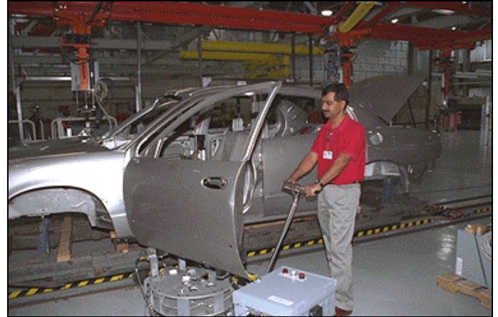
Figure 6. The cobot door unloader (courtesy of General Motors Company).
